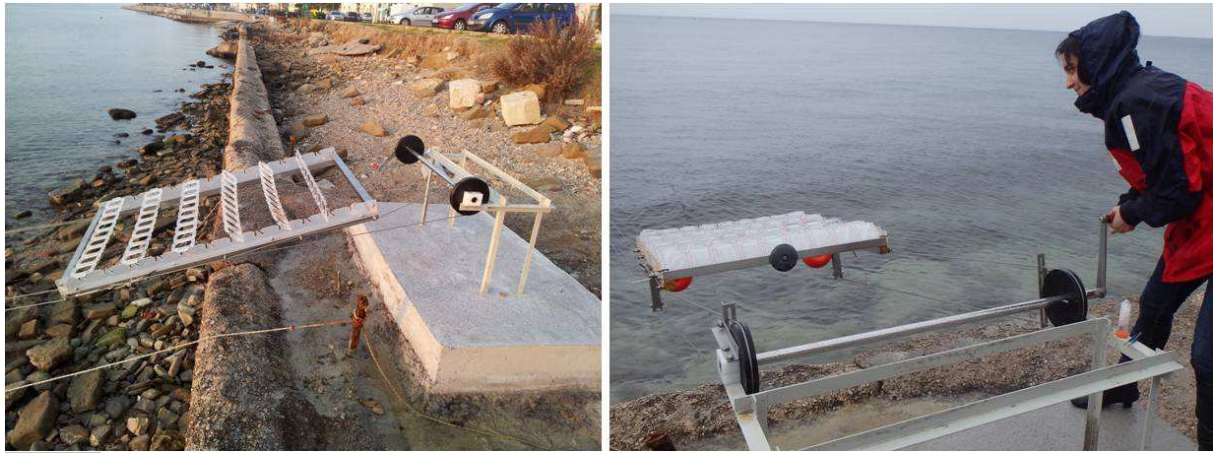
Figure 4: The exclusively made cableway with a special holder for experiments in the sea
